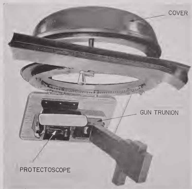
FIGURE 7. Inside view of model of rear turret machine gun mount.
